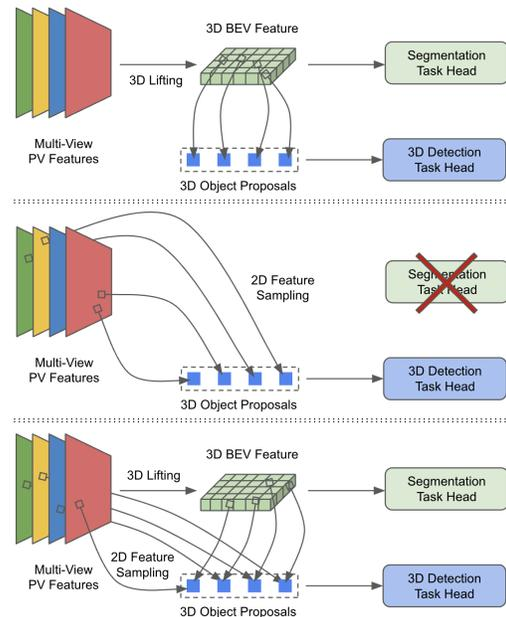
Figure 1. Comparison of different image-only 3D perception frameworks. **(a) Top:** Bird’s-eye-view-based (BEV-based) methods **(b) Middle:** Perspective-view-based (PV-based) 3D detection-only methods **(c) Bottom:** DuoSpaceNet (ours) where 3D detection benefits from both 3D BEV and 2D PV feature space. Dense segmentation is also doable.
