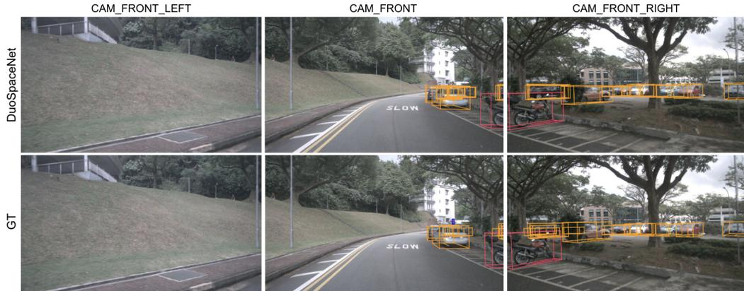
Figure 6. Visualization of 3D detection results in perspective camera view. Different colors represent different categories.
