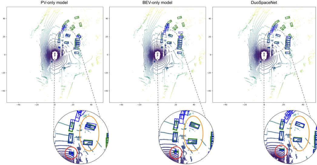
Figure 5. Visualization of 3D detection results in top-down view. Ground truth bounding boxes are in green and predictions are in blue
