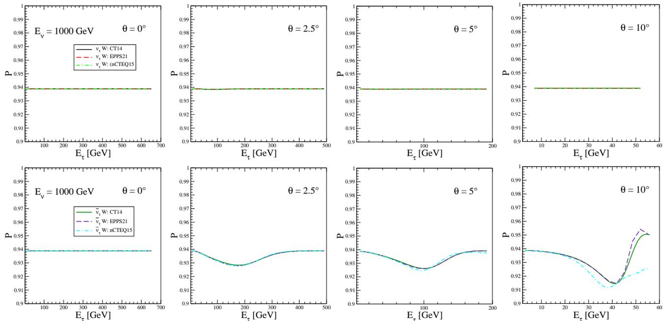
FIG. 7: Degree of polarization of the tau (upper panels) and antitau (lower panels) produced in  $\nu_\tau W$  and  $\bar{\nu}_\tau W$  interactions, respectively, as a function of the tau lepton energy for an incident (anti) neutrino with an energy of 1000 GeV. Results for different values for the angle  $\theta$  derived assuming distinct nPDFs.
