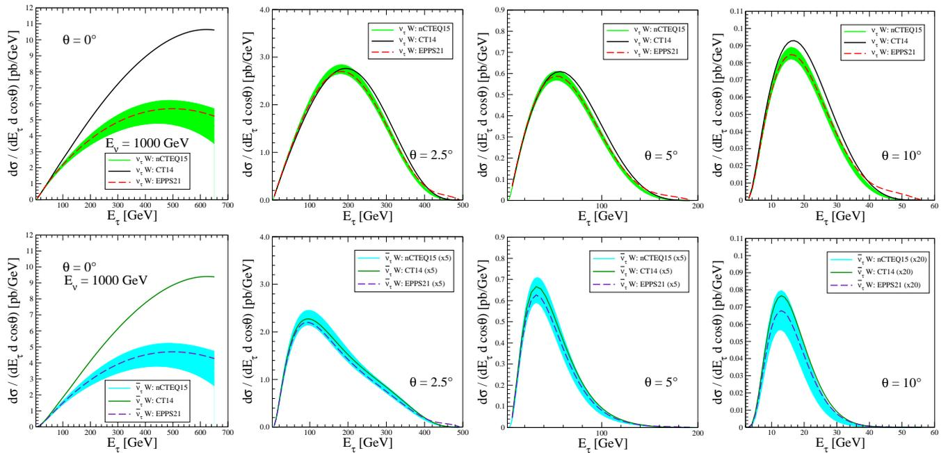
FIG. 4: Double differential  $\nu_\tau W$  (upper panels) and  $\bar{\nu}_\tau W$  (lower panels) cross-sections as a function of the tau lepton energy for different values of the angle  $\theta$ . Results derived assuming different nPDFs and that the energy of the incoming tau neutrino is equal to 1000 GeV. Note the different  $y$ -axis scales in the distinct plots.
